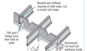
2x4 block for soffit support
