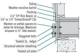
Maintain 2" distance (minimum) from edge of ledger to edge of fastener. Stagger bolts.
