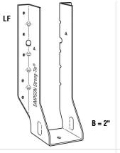
LF – 18 gauge The LF series features fast and easy installation. No web stiffeners required. Has uplift factored resistance of 110 lb.
