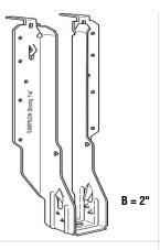
IUS - 18 gauge The IUS is a hybrid hanger that incorporates the advantages of face-mount and top-flange hangers. Joist nails are not required. Has uplift factored resistance of 105 lb.
