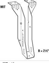
MIT – 16 gauge The MIT's positive-angle nailing helps minimize splitting of the I-joists' bottom flange. Has uplift factored resistance of 375 lb.
