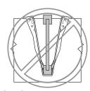
Hanger Over-Spread Hanger over-spread can raise the I-Joist above the header and may cause uneven surfaces and squeaky floors.
