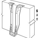
STEP 1 Attach the ITS to the header
