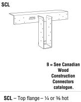
SUL – Top hange – 1/4 of 3/6 not rolled angle Stirrup – 3 gauge This series offers high load capacities. The large top flange distributes the load to the carrying member.
