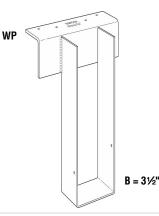
WP - Top flange - 7 gauge; Stirrup – 12 gauge This welded series offers the greatest design flexibility and versatility, and a large selection of sizes. Suitable for welded and nailer applications, and modifications including slopes and skews. No uplift resistance.
