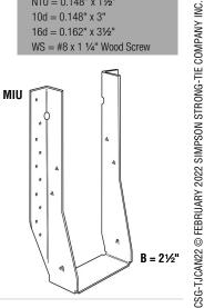
MIU - 16 gauge The MIU series features 16gauge steel and extra nailing for higher loads. Has uplift factored resistance of 375 lb.
