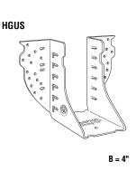
HGUS – 12 gauge HHUS – 14 gauge Features double shear nailing for high strength and lowest installed cost due to the reduced nail quantity requirement. Not suitable for use with l-joists.
