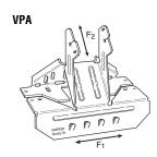
VPA-18 gauge This variablepitch connector allows a sloped beam to sit on a top plate without having to notch, birdmouth, bevel, or toe nail. It also provides uplift capacity. Adjustable from 3:12 to 12:12 pitch.
