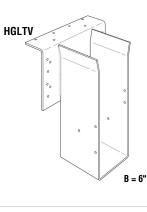
HGLTV – Top flange – 3 gauge Stirrup – 7 gauge This welded series provides high load carrying capacity and design flexibility and versatility. May be sloped, skewed and modified in other ways, and may be welded to steel Ibeams.
