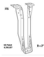
ITS - 18 gauge The ITS top-flange hanger with its Strong-Grip™ seat and Funnel Flange™ installs faster than any other top-flange hanger. Joist nails are not required. Has uplift resistance of 105 lb.
