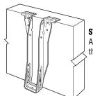
**STEP 1**Attach the ITS to the header
