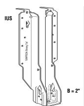
IUS - 18 gauge The IUS is a hybrid hanger that incorporates the advantages of both face-mount and top-flange hangers. Joist nails are not required. Has uplift resistance of 60 lb.
