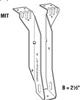
MIT – 16 gauge The MIT's positive-angle nailing helps minimize splitting of the I-joists' bottom flange. Has uplift resistance of 215 lb.
