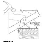
**STEP 2**Seat rafter with a hammer, adjusting "B" flange to the required pitch.
