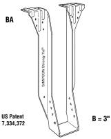
**BA** – 14 gauge The BA is designed especially for use with multiple ply headers 1½" to 1¾" thick, and may be used for weld-on applications. Has uplift resistance of 1050 lb.
