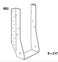
MIU – 16 gauge The MIU series features 16 gauge steel and extra nailing for higher loads. Has uplift resistance of 200 lb.
