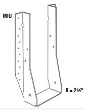
MIU - 16 gauge The MIU series features 16gauge steel and extra nailing for higher loads. Has uplift resistance of 210 lb.
