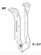
MIT - 16 gauge The MIT's Positive Angle Nailing helps minimize splitting of the I-joist's bottom flange. Features uplift capacity and extended seat design (to allow installation of slightly undercut joists). Has uplift resistance of 185 lb.
