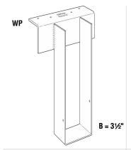
WP – Top flange – 7 gauge; Stirrup – 12 gauge This welded series offers the greatest design flexibility and versatility, and a large selection of sizes. Suitable for welded and nailer applications, and modifications including slopes and skews. No uplift resistance.
