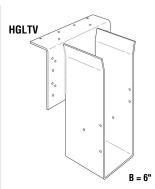
**HGLTV** – Top flange – 3 gauge Stirrup – 7 gauge This welded series provides high load carrying capacity and design flexibility and versatility. May be sloped, skewed and modified in other ways, and may be welded to steel Ibeams.
