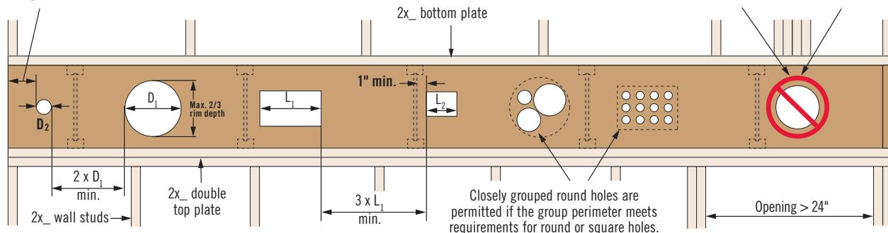
**Do not locate holes under concentrated loads such as, trimmers or columns**
