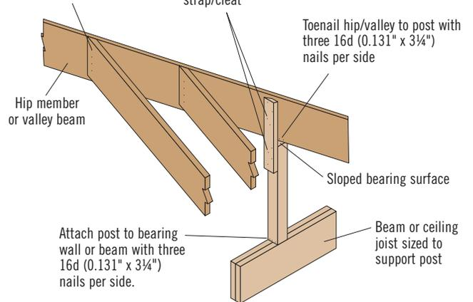
Attach post to bearing wall or beam with three 16d (0.131" x 3/4") nails per side.
