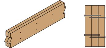
Multiple pieces can be nailed or bolted together to form a header or beam of the required size, up to a maximum width of 5¼". Load must be applied evenly across entire beam width.
