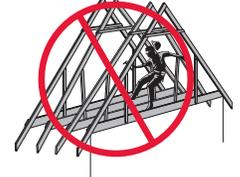
DO NOT walk on joists or rafters until braced. INJURY MAY RESULT.
