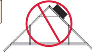
DO NOT stack building materials on unsheathed joists or rafters.
