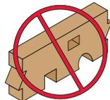
**DO NOT cut, notch, or drill holes in rafters, ceiling joists, hips, or valleys except at birdsmouth cut locations or as indicated in the illustrations and tables above.**
