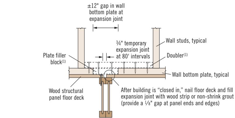
(1) Install plate filler block and doubler to splice bottom plate after floor deck is nailed and building is “closed in.”
