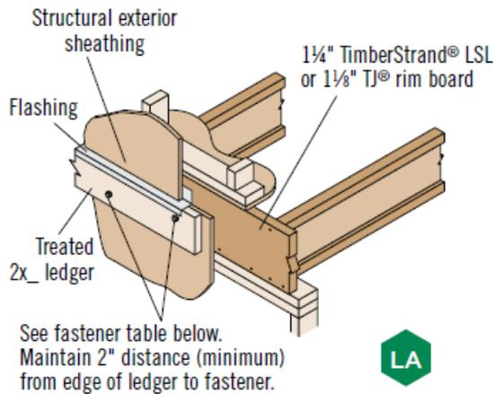
**Treated deck ledgers must be properly flashed to ensure rim board is protected from moisture and ensure connections perform.**
