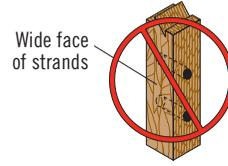
DO NOT install bolts or screws into the narrow face of strands
