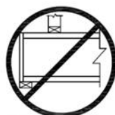
Uniform loads only—no offset bearing walls
