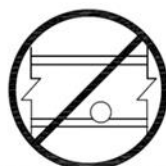
Hole must only be located in web—do not cut flange
