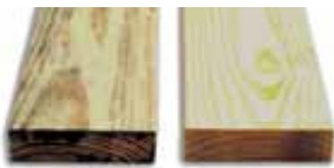
**Untreated lumber (at left) exposed to moisture can become a costly problem. Lumber protected with an effective anti-mold and anti-sapstain solution (at right) combined with good inventory control practices addresses this problem.**
