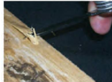
Pick test on sound wood—splintering break
