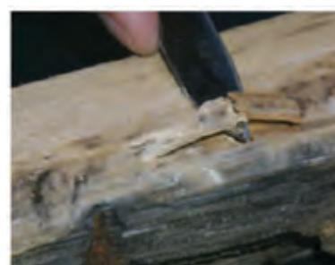
Pick test on decayed wood—brush break
