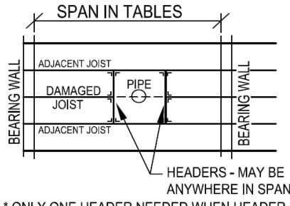
\* ONLY ONE HEADER NEEDED WHEN HEADER OCCURS WITHIN 12" OF BEARING WALL
