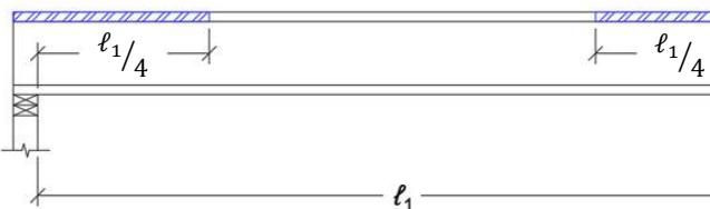
= Location Zone for Side Flange Notch between End Bearing and Quarter-Span
