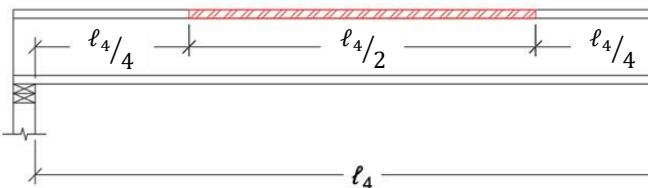
= Location Zone for Side Flange Notch between Quarter-Span and Mid-Span
