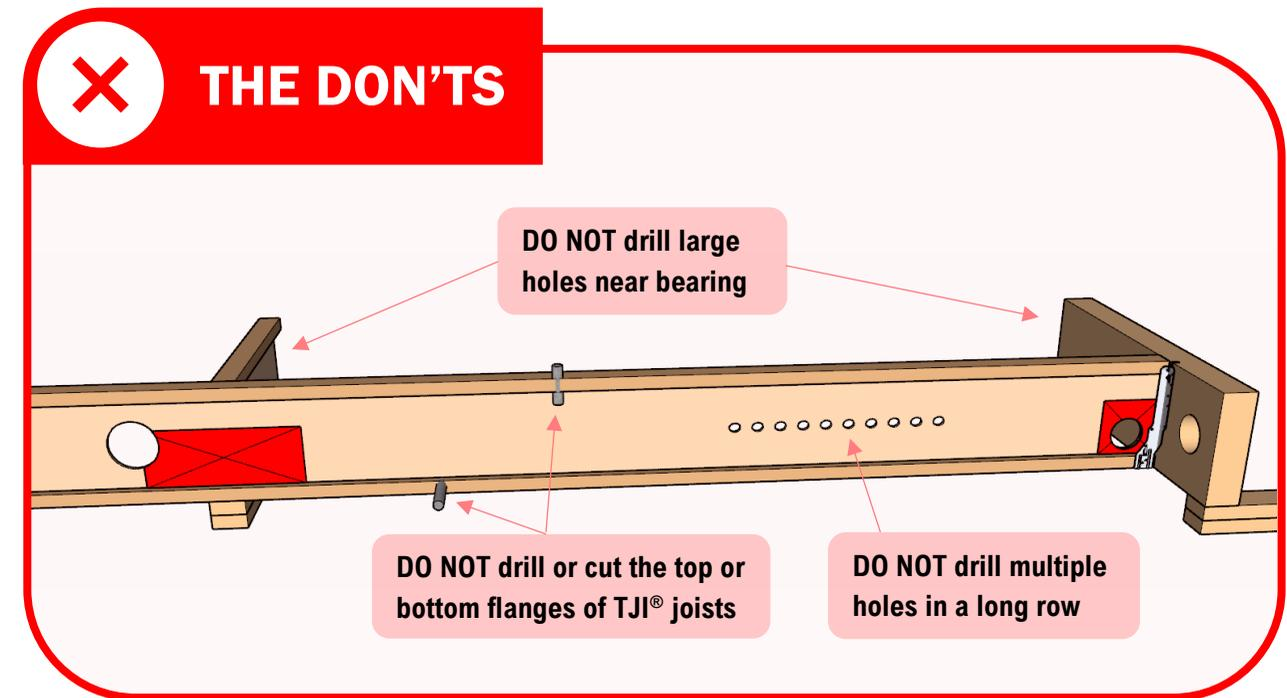
Review hole placement/size using the [Trus Joist Allowable Hole Chart \(TJ-9015\)](#)
