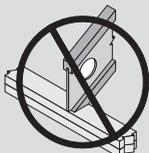
DO NOT cut holes too close to support. Refer to Allowable Holes on page 1 for minimum distance from support.
