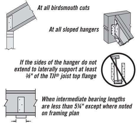
**W** \* With a point load from above and no support below, install web stiffener tight to top flange (gap at bottom flange)
