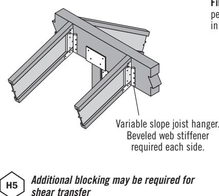
Filler block: Attach per table in detail H2 in floor section of guide.
