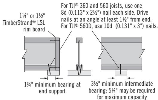
Shear transfer nailing: At minimum, use connections equivalent to floor panel nailing schedule
