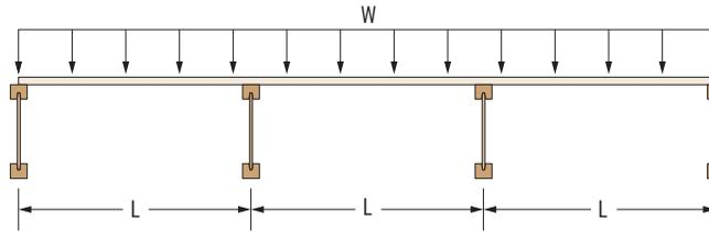
The equations above are based on one-way "beam" action. They are provided to help develop allowable uniform loads based on moment, shear, and deflection as applied to one-, two-, and three-span conditions. Loads derived from the equations provided are assumed to be applied over full-size panels in normal sheathing applications. The following definitions apply:
