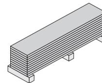
Store and handle Parallam® PSL, Microllam® LVL, and TimberStrand® LSL in flat orientation (wrapped)
