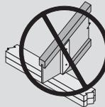
DO NOT overhang birdsmouth cut from inside face of plate. TJI® joist flange must bear fully on the plate.
