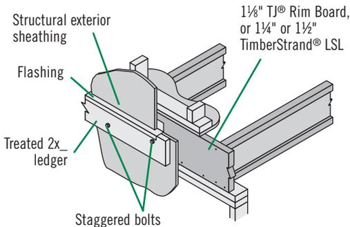
**LA** Corrosion-resistant fasteners required for wet-service applications
