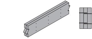
**L6** Multiple pieces can be nailed or bolted together, up to a maximum width of 7"
