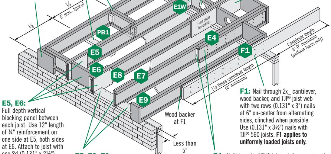
**E5, E6:** Full depth vertical blocking panel between each joist. Use 12" length of  $\frac{3}{4}$ " reinforcement on one side at E5, both sides at E6. Attach to joist with one 8d (0.131" x 2½") nail at each corner.
