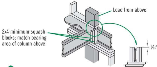
**CS** Use 2x4 minimum squash blocks to transfer load around TJI joist
