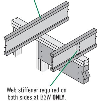
**B3 B3W** *Blocking panels may be required in Seismic Design Categories D<sub>0</sub>, D<sub>1</sub>, and D<sub>2</sub> and/or with braced/shear walls above or below—see detail B1*
