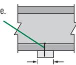
3½" minimum intermediate bearing; 5¼" may be required for maximum capacity
