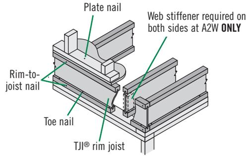
**A2** **A2 W** Must have 1 1/4" minimum joist bearing at ends. Attach rim joist per A3.1 in rim board installation table above.
