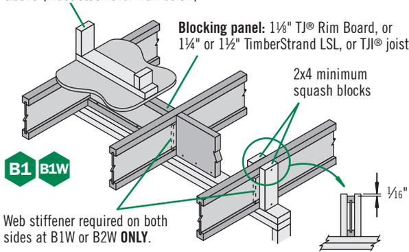
**B2 B2W** *Blocking panels may be required in Seismic Design Categories D<sub>0</sub>, D<sub>1</sub>, and D<sub>2</sub> and/or with braced/shear walls above or below—see detail B1*
