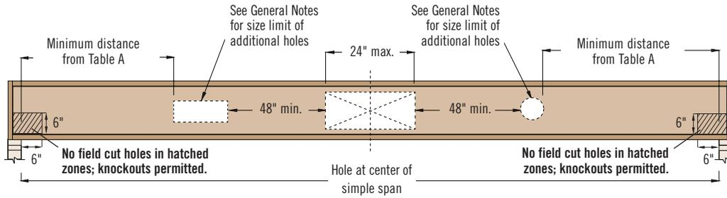
Maximum Hole at Mid-Span for TJI® 360 and TJI® 560 Joists
