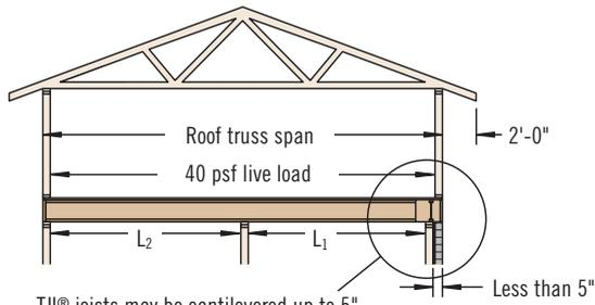
TJI® joists may be cantilevered up to 5" when supporting roof load, assuming:
