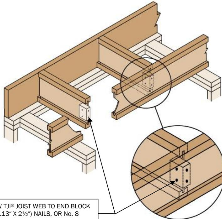
[TYP] NAIL OR SCREW TJI® JOIST WEB TO END BLOCK WITH TWO (2) 8d (0.113" X 2½") NAILS, OR No. 8 WOOD SCREWS (LENGTH = 2½")
