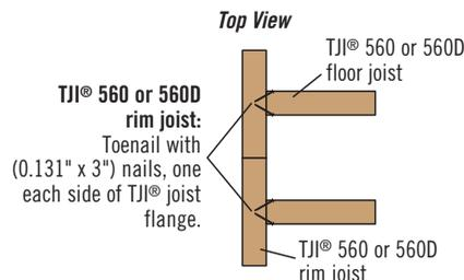
Locate rim board joint between joists
