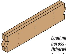
Load must be applied evenly across entire beam width. Otherwise, use connections for side-loaded beams
