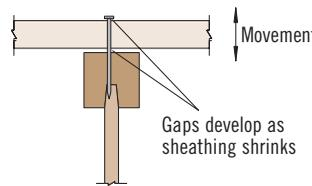
Keep building materials dry, and properly glue floor panels to the joists. Panels that become excessively wet during construction shrink as they dry. This shrinkage may leave gaps that allow the panel to move when stepped on.
