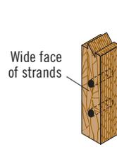
In order to use the manufacturer's published capacities when designing column caps, bases, or holdowns for uplift, the bolts or screws must be installed perpendicular to the wide face of strands as shown at left.
