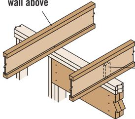
Web stiffeners required on both sides at B3W ONLY. See footnote (1) under span tables.
