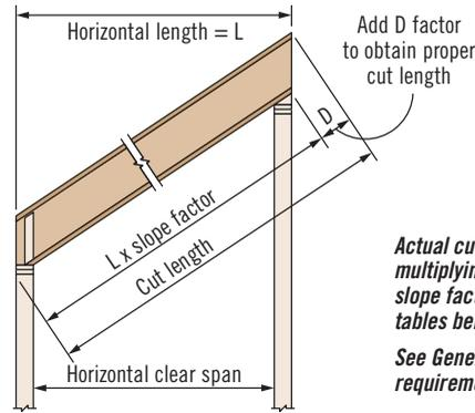
Actual cut length can be approximated by multiplying the horizontal length by the slope factor and adding the D factor. See tables below.
