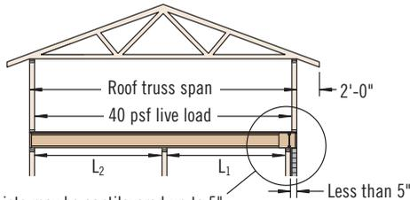
TJI® joists may be cantilevered up to 5" when supporting roof load, assuming:
