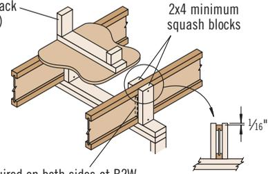
Web stiffeners required on both sides at B2W ONLY. See footnote (1) under span tables.
