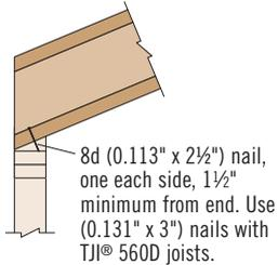
*When slope exceeds 1/4:12, a beveled bearing plate, variable slope seat connector, or birdsmouth cut (at low end of joist only) is required.*
