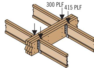
First, check allowable load tables on pages 6–23 to verify that three pieces can carry the total load of 715 plf with proper live load deflection criteria. Maximum load applied to either outside member is 415 plf. For an assembly of three 1¾" plies (Assembly B), two rows of (0.131" x 3") nails on both faces at 12" on-center are good for only 280 plf. Therefore, use three rows of (0.131" x 3") nails on both faces at 12" on-center (good for 420 plf).
