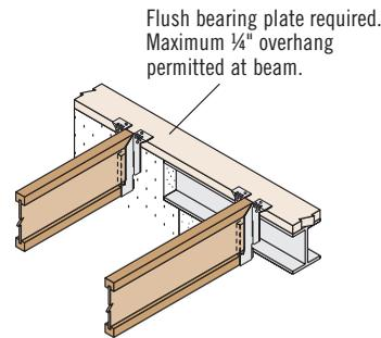
Flush bearing plate required. Maximum ¼" overhang permitted at beam.
