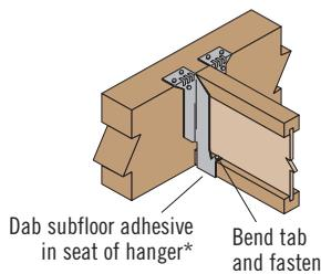
Seat the joist tight to the bottom of the hanger. When using hangers with tabs, bend the flange tabs over and nail to the TJI® joist bottom flange. Placing a dab of subfloor adhesive\* in the seat of the hanger prior to installing the joist can reduce squeaks.
