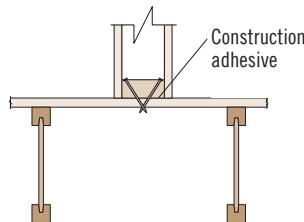
Nail interior partitions to the joists when possible. If the wall can be nailed only to the floor panel, run a bead of adhesive\* under the wall and either cross nail, nail through and clinch tight, or screw tightly into the wall from below.
