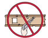
**DO NOT cut holes in cantilever reinforcement.**
