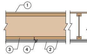
1. 48/24 tongue-and-groove, span-rated sheathing (Exposure 1), glued with a subfloor adhesive and nailed
