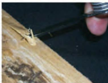
Pick test on sound wood—splintering break
