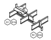
For TJI® joists which bear on an intermediate support below and support an interior bearing wall above, Weyerhaeuser requires blocking to be installed at the intermediate support (see detail B1). If the walls above and below are <u>not shear walls</u>, squash blocks may usually be substituted for blocking panels (detail B2) with the approval of the Designer of Record.
